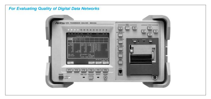
Bit error rate measurement is the most critical parameter in evaluating the quality of digital transmission modes. However, conventional methods, which measure only average bit error rates, are inadequate. In the MD6420A, various types of extension and remote control units are provided as options, as well as units which allow the use of various types of interfaces.
